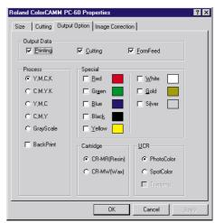
Make sure to always select [FormFeed] when printing tile page. And if there is cutting data, select [Cutting] and set the suitable [Process] depending on data.
